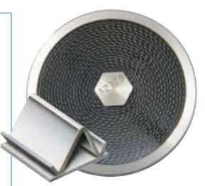
After more than 70 years of manufacturing and testing experience, Amal has conclusive proof that a crimped metal design of triangular cells is the most effective method of quenching potentially lethal or destructive flames. They can be used on all Gas Groups, i.e. IIA, IIB and IIC to EN50014, as well as B, C and D to US National Electrical Code Article 500.
