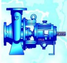
Process centrifugal pump to ISO-5199 "upgraded medium duty". NQ series with dimensions to ISO-2858. For high temperature, version NQT in "centerline" layout. Closed or semi-open impeller, it is possible to include an inducer for low NPSHr. Oil-lubricated bearings. Sealing by mechanical seal with various API plans. For pumping clean or agressive fluids or with solid particles. Process design: removal of rotor without remove pump casing nor motor (back pull-out).
