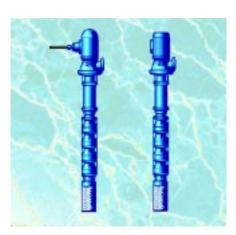
Vertical turbine pump for deep well. Multistage with closed impellers, column section with bearing, shat sleeve, discharge head sealing by packing and driven by electric motor, diesel engine or tractor. For pumping clean or agressive fluids, not containing abrasive or solid particles.
