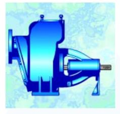
Self-priming horizontal centrifugal pump. Wide width of open or semi-open impeller, with wear plate. Sealing by mechanical seal. For pumping clean or agressive fluids or with solids particles.
