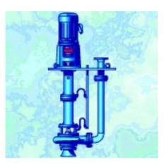
Non-clogging centrifugal vertical sump pump, for dry or wet well installation. Vortex or semi-open or two/three channels impeller. Fitted with delivery pipe up to support plate (RWCP), or without delivery pipe (RWCN). Close-coupled version IFV series with vortex impeller. For pumping clean or agressive fluids or with a high solids content.
