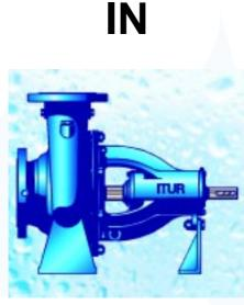
Centrifugal pump to DIN-24255, and extension range with complementary sizes. Closed impeller. Sealing by mechanical seal or packing. For pumping clean, slightly agressive fluids, not containing abrasive or solid particles. Process design: removal of rotor with pump casing and motor in situ (back pull-out).
