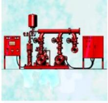
Fully Automatic Fire-fighting Equipment and System, composed by jockey pump and one or several service pumps, with electric motor or diesel engine. Its include collector, valves, accesories and electrical panels. According to the Standars UNE-23500/90, Cepreven RT2-ABA/96, NFPA-20, etc. For pumping clean water or seawater.
