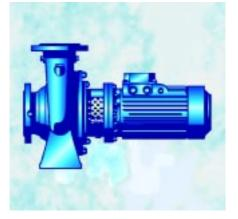
Centrifugal close-coupled electric driven pump, based on DIN-24255. Closed impeller. Sealing by mechanical seal. Standard I.E.C. motor. For pumping clean, slightly agressive fluids, not containing abrasive or solid particles.
