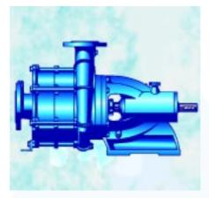
Horizontal multistage centrifugal pump, ball-bearing support and suction guidebearing. Closed impellers. Sealing by packing. For pumping clean fluids, not containing abrasive or solid particles.
