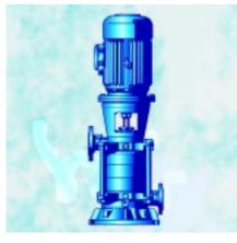
Vertical multistage centrifugal electric driven pump. Closed impellers. Sealing by mechanical seal. Standard I.E.C. motor. For pumping clean, slightly agressive fluids, not containing abrasive or solid particles.
